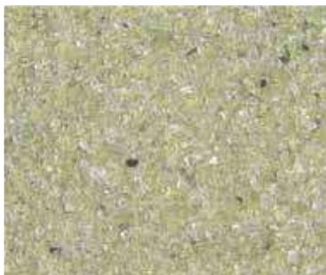
Crushed glass is effective for removing surface contaminants, paint, rust and coatings from a variety of substrates, including metal, concrete and wood, while producing a relatively low dust profile and a consistent finish. Waste, recycled glass product. **Available in various mesh sizes.**
